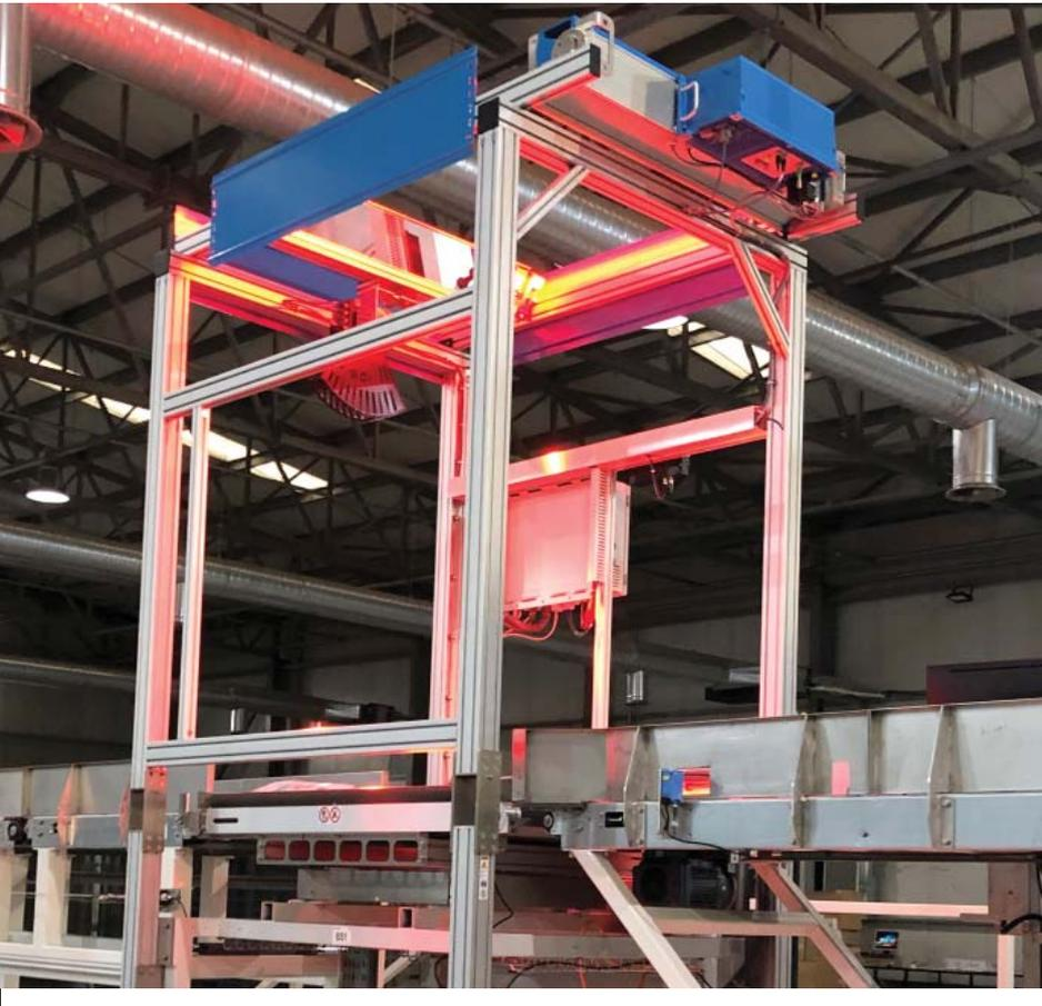
DWS system for measuring weight and dimensions, as well as save photos of items passing through.
