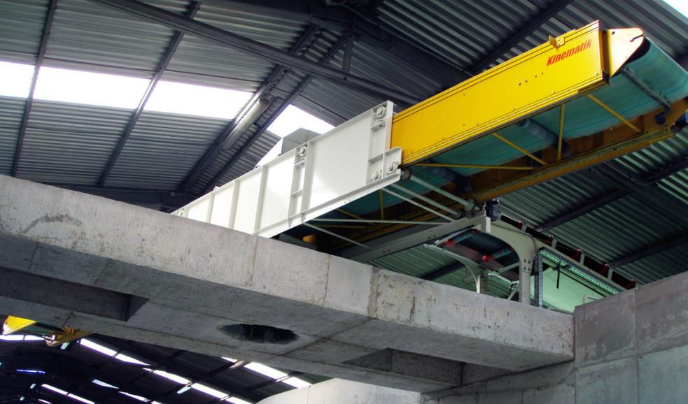
Telescopic and rotating conveyor for storing fertilizer.
